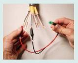
GREEN LED means wiring is properly identified.
